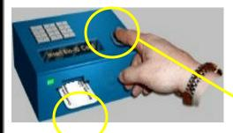
Insert the card and touch the panel. The software decodes the  $VSCODE^{\text{TM}}$  to compare with your fingerprint on the panel.
